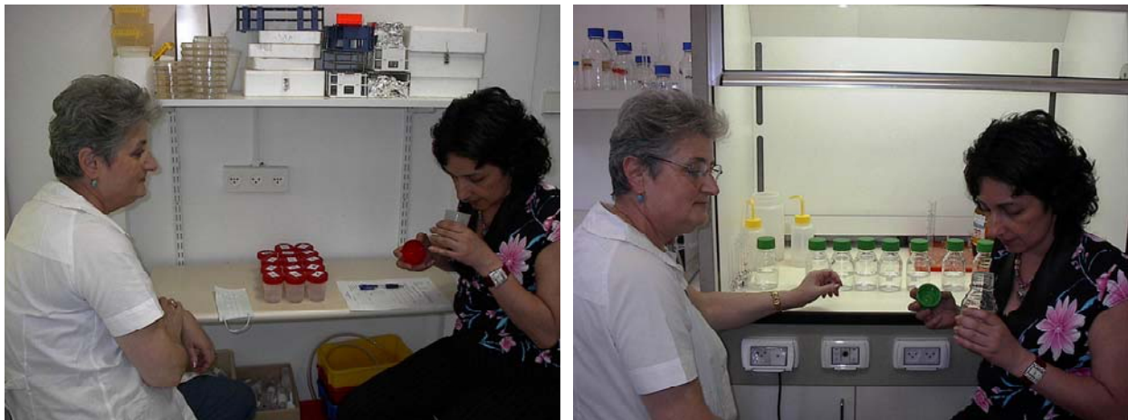
Figure 1. Left: A triangular forced-choice test (actual tests are performed with wide-mouth glass bottles). Right: Odor intensity evaluation.
